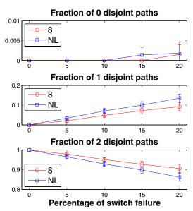
Figure 5: Scafida tolerates the failure of switches well; the impact of node failures on the number of disjoint paths is shown
