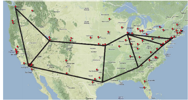
Figure 1: Abilene backbone and PlanetLab sites using Abilene. lead to lower application performance. Clearly, this inefficiency could be avoided by choosing low-latency or small hop-count peerings, and the resulting locality could reduce the network load as each connection would traverse fewer backbone links.
