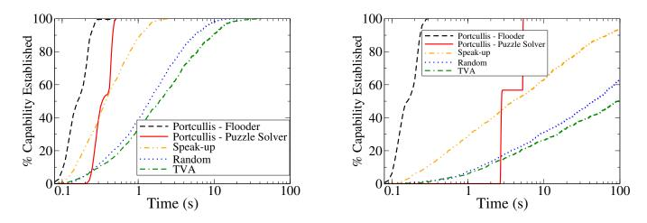
Figure 4: Capability Setup Time. Cumulative distribution functions of the time required for a legitimate sender to acquire a capability when faced with 1,000 attackers (left) and 20,000 attackers (right). The Portcullis Puzzle Solver attacker uses the optimal strategy discussed in Section 6.2. Note that the x-axis uses a logarithmic scale.
