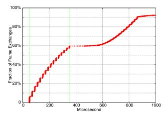
Figure 4: Access delay  $(d_{t0})$  distribution of one hour of head-of-line blocked frame exchanges from an Avaya AP-8 AP to a client doing a bulk TCP download.
