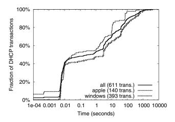
Figure 14: Distribution of DHCP transaction durations for an entire day.
