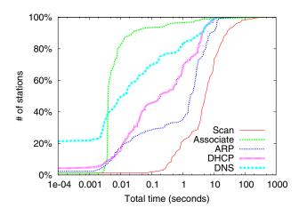
Figure 12: CDF of time spent in each successful phase of startup.
