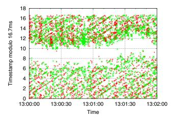
Figure 1: Physical error frame pattern during microwave oven use. The y-axis depicts (time % 16) ms, showing the offset of physical error packets within the 16 ms microwave period. The x-axis shows two minutes of microwave use.
