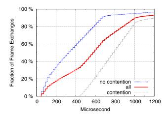
Figure 5: Access delay  $(d_{t0})$  distribution of head-of-line blocked frame exchanges from a Cisco Aironet 350 AP to a client doing a bulk scp download.
