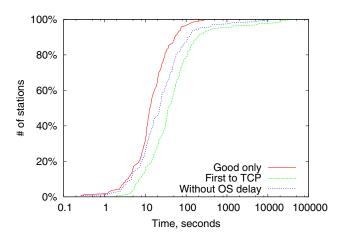
Figure 11: CDF of the delay experienced on startup by 802.11 clients in our network.
