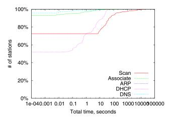
Figure 13: CDF of delays experienced by 802.11 clients due to timeouts.
