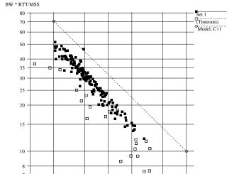
Figure 10: Measured TCP data, Set 1 This data fits Equation 3 with  $C=0.700\pm0.057$  or to Equation 5 with k=-0.525,  $C=0.574\pm0.045$ . These values for C are about 25% lower than TCP in a simulator.
