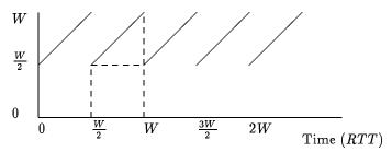
Figure 1: TCP window evolution under periodic loss Each cycle delivers  $(\frac{W}{2})^2 + \frac{1}{2}(\frac{W}{2})^2 = 1/p$  packets and takes W/2 round trip times.
